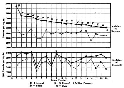
Fig. 20.—Effect of "boiling process" of preservative treatment on the strength and stiffness of Douglas-fir stringers treated green, air seasoned and tested.
